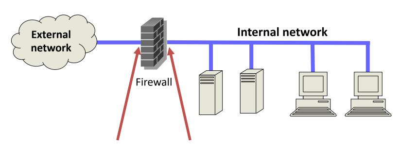
Firewall has two network interfaces: One for external traffic, one for internal traffic
